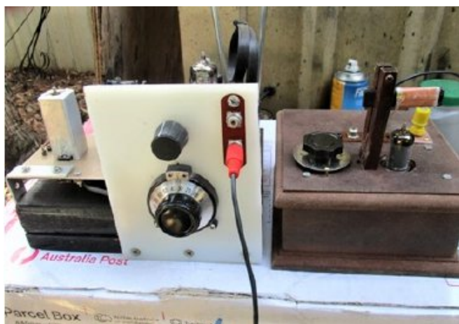
AM Modulator in use with my home-made FM tuner
