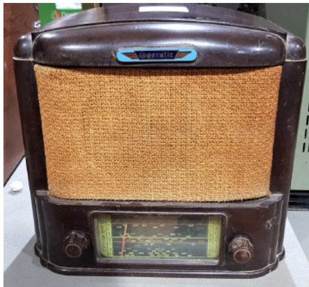
Philips Operatic 37MA bakelite, 4-valve, MW, AC mantle radio made in Australia 1947
