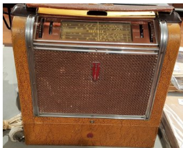
A Breville portable battery-AC leather-wrapped timber case radio, model 857, 1949, broadcast band, 5 valve, Superhet with RF stage, made in Australia.
