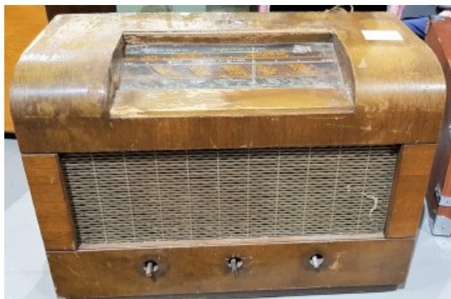
HMV model 1120 radio, MW/LW/SW, wooden case, 5-valve, AC mantle radio made in UK in 1949, was auctioned.
