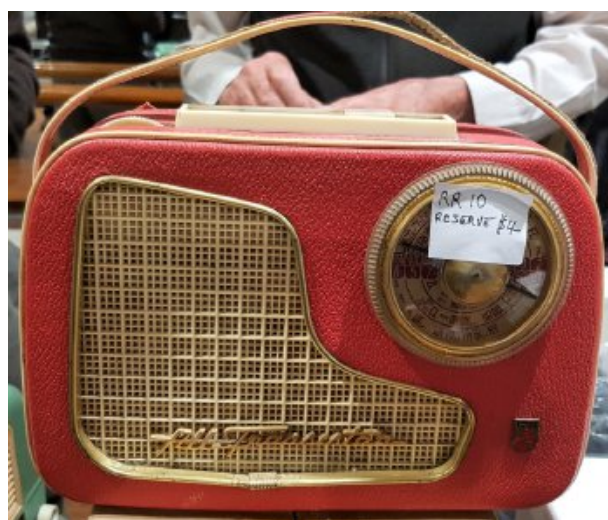
Philips Radioplayer All Transistor 199, portable 7-transistor, 9v battery made in Australia 1959/1960, original price 44 Aust. Pounds (seems expensive!)
