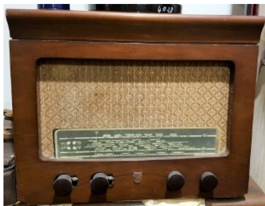
Philips Table Radiogram 532A 5-valve SW/MW/LW , manual turntable, wood cabinet, Made in UK 1954?
