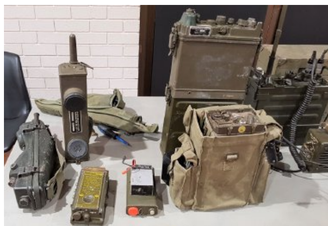
From left to right: Transceivers—PRC-6 (Korea); At rear- BC-611 (WW2); URC-4 emergency vhf/uhf and battery pack; At back- PRC-10 (Vietnam); At front- Canadian CPRC-26 (Korea); PRC-77 solid state transceiver (Vietnam)
