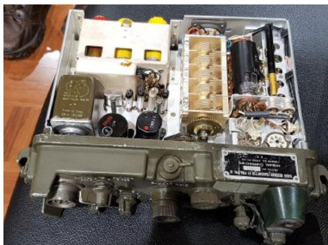
Inside the PRC-10 (Vietnam) -minaturised components (see pencil valves) and chassis !960's for rugged portable applications in a wartime situation.
