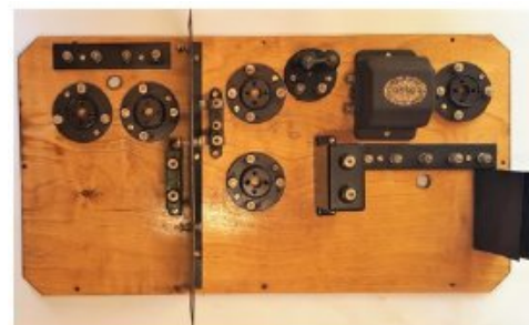
All bakelite parts were cleaned and mounted to the chassis.
