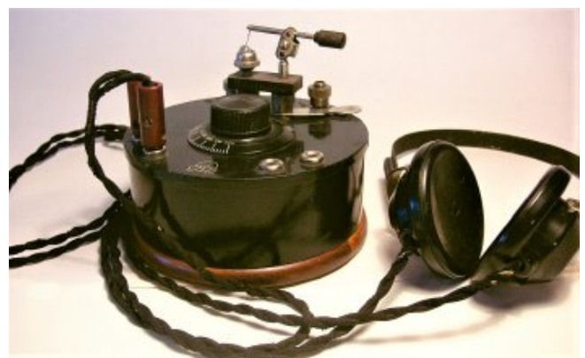
Radiola crystal set c.1922 (Sweden) with earphones and cat’s whisker detector. .
