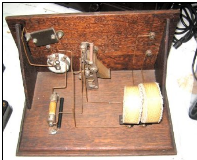
A carborundum crystal detector
