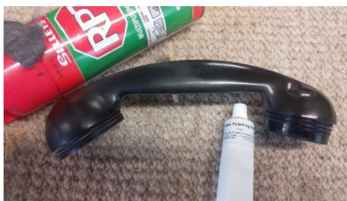
L-R: 1. Degraded Bakelite surface. 2. Left half RP7 and steel wool only, right half finished with polishing paste and buffed
