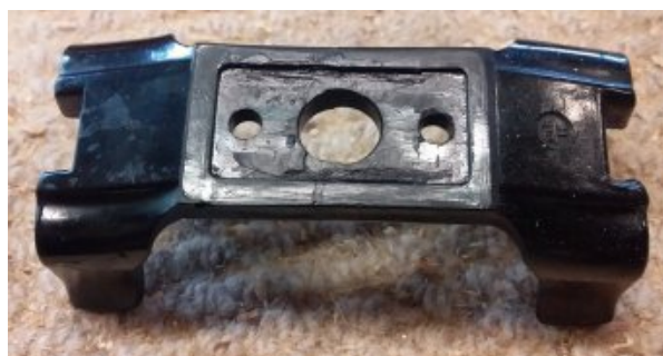
Two Bakelite cradle halves epoxy glued and stitched underneath
